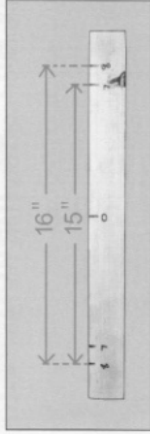
Figure 4. 2X4 wall block spacing tool. This simple-to-make tool accurately spaces the wall blocks.
